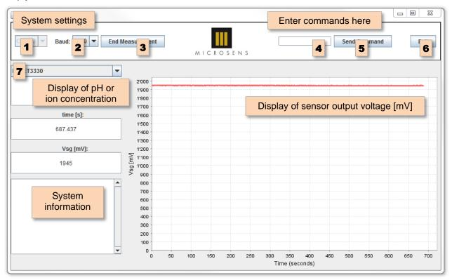
Once the measurement file is selected the graphical user interface will open, as shown in the above picture. In order to connect to the MSFET3330 Interface, the user needs to select the corresponding COM port (1). The baudrate should be set to 4800 for a correct communication between the PC and the MSFET3330 Interface (2). Clicking on "Start Measurement" (3) will start the measurement and the received data will be displayed.
