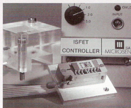
DIL packaged ISFET multi-sensor device for flow through measurement
